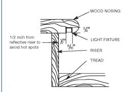
Custom fabricated fixtures are manufactured to the exact dimension required. Each LED fixture is built with an 18" lead wire from one end.
