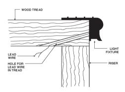
Custom fabricated fixtures are manufactured to the exact dimension required. Each LED fixture is built with standard 18" lead wires from one end.
